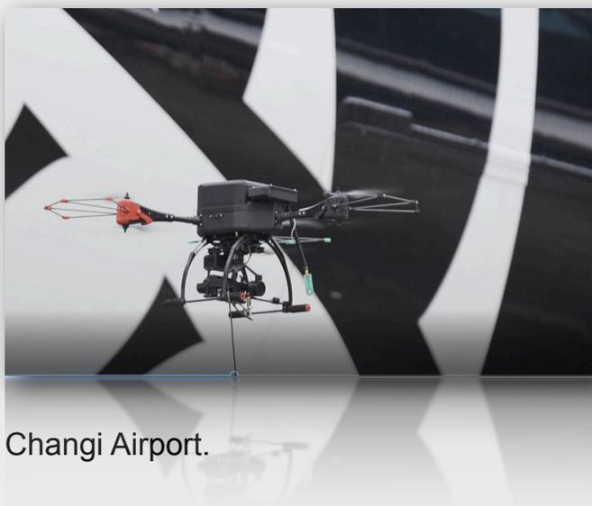
It is here AirNZ planes undergo heavy maintenance checks and the unmanned drones developed by ST Engineering are doing a job **that would previously be performed** by an engineer on a boom lift.
